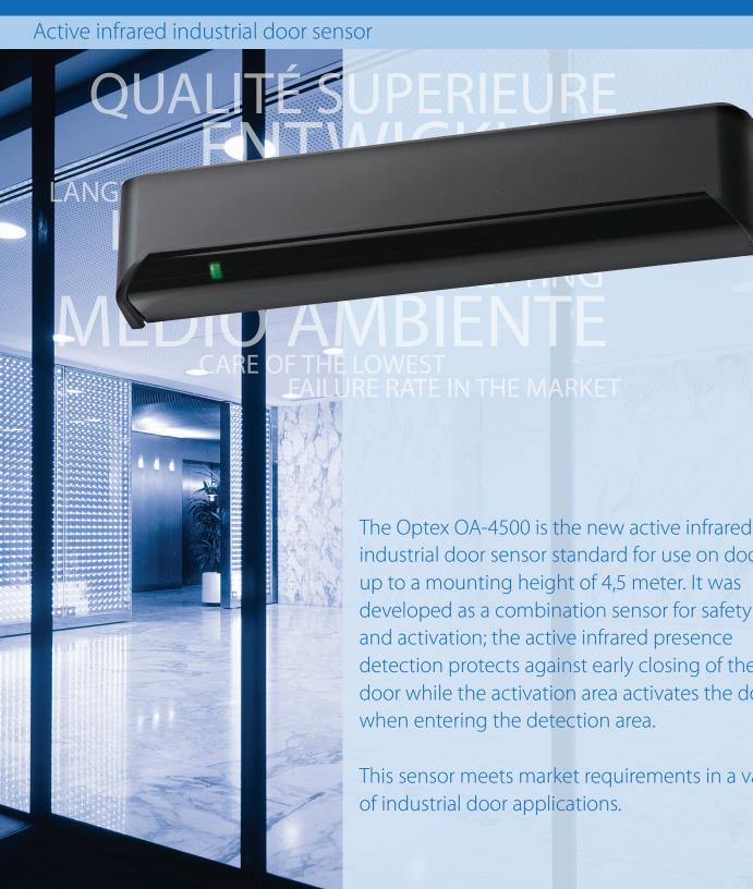
industrial door sensor standard for use on doors up to a mounting height of 4,5 meter. It was developed as a combination sensor for safety and activation; the active infrared presence detection protects against early closing of the door while the activation area activates the door
